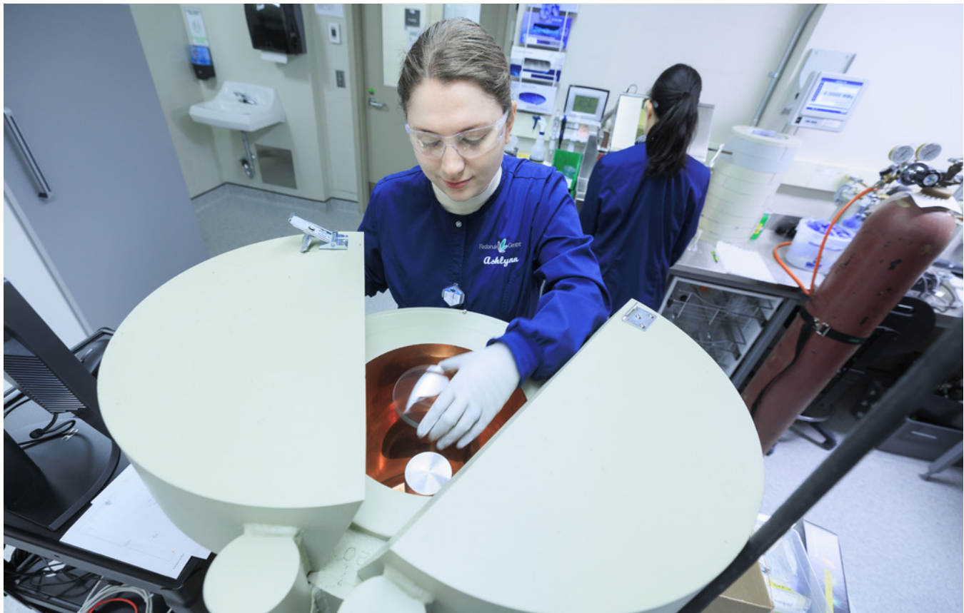
Figure 2 - A Fedoruk Centre Technologist loads a sample into the high-purity germanium gamma spectrometer.
