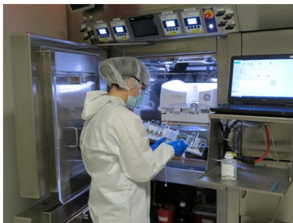
Figure 3 - Radiopharmaceuticals are manufactured with automated chemical equipment inside hot cells that protect employees from radiation. Employees dress to ensure the product is sterile for clinical applications.
