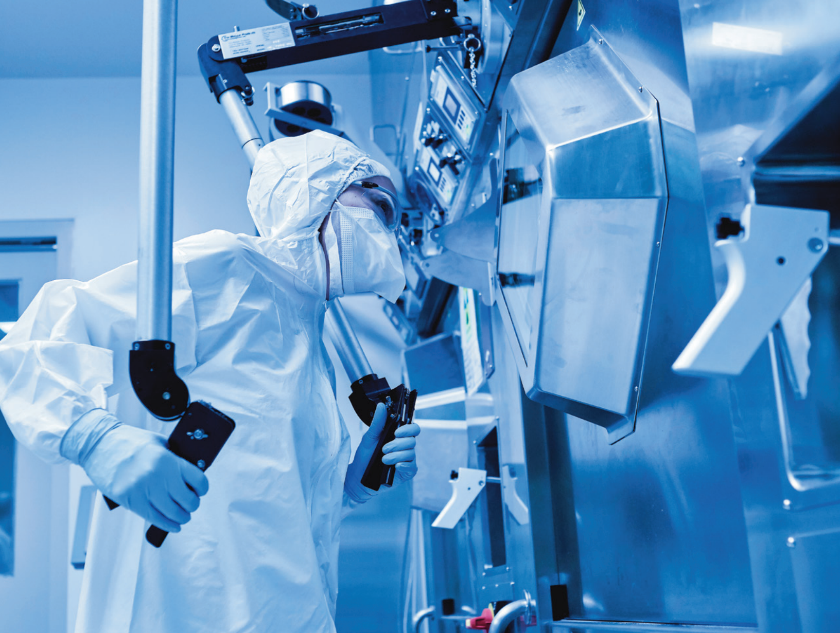
Fedoruk Centre Production Technologist using robotic arms in the hot cell room during the manufacture of FDG, a radiopharmaceutical produced daily for clinical PET-CT imaging.
