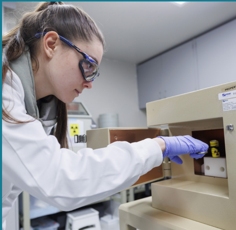
Researchers use instruments such as a gamma spectrometer to characterize radiological samples.
